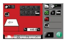
Using the screen is simplicity itself. Key in the sheet length (popular sizes are pre-set), touch the fold type for the finished product (letter, gate etc) and press the green button. The AutoCreaser Pro 33 will automatically
