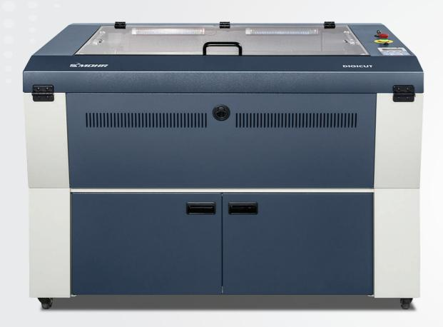
Digicut opens up a wide variety of creative possibilities for the processing of a single sheet. Using laser you can not only cut sophisticated designs, but also punch, engrave and crease – all in one pass; and this on variety of different materials. There are almost no limits in terms of design. Also not tooling costs arise by the use of a laser.
